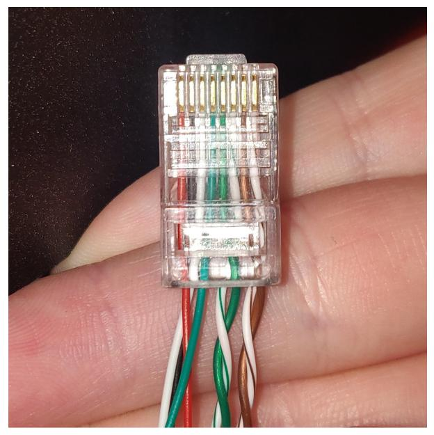
Make sure that all wires are fully inserted in the connector before you crimp it, but also ensure that no part of the wires extend through the connector if your connector does not stop wires from going through the entire assembly.
